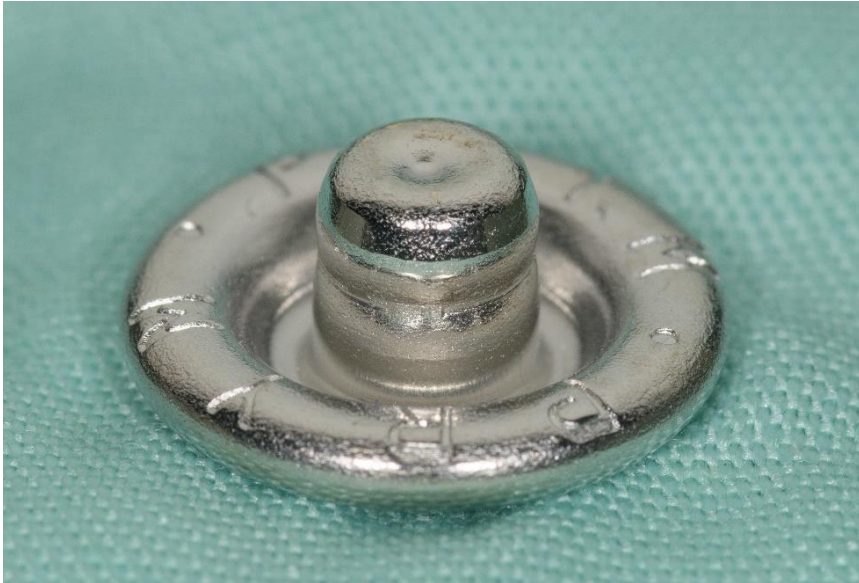
Male fastener part for the Philip badge/hat before testing showing no wear
