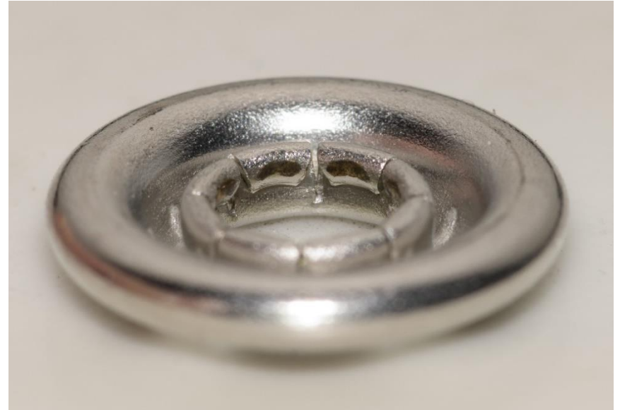
Female fastener part for the Philip badge/hat after testing showing slightly polished contact area
