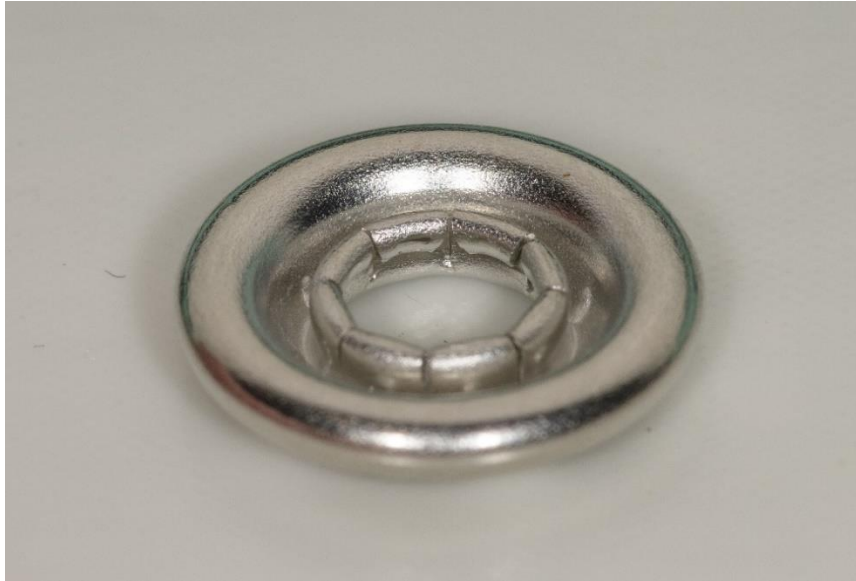
Female fastener part for the Philip badge/hat before testing showing no wear
